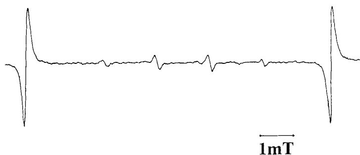
FIGURE 5 The ESR spectra of the spin adducts of \cdot\text{OH} observed under a dark condition. The ESR spectra of the Chlorella vulgaris solution was measured by ESR under a dark condition with DMPO after 80,000 lux of visible light was irradiated for 20 min without DMPO.
